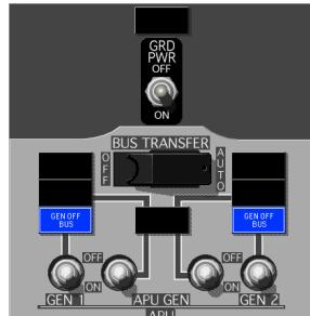
If SOURCE OFF lights do not extinguish, battery power is the only source. Land at the nearest suitable airport.
